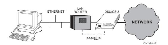
Figure 2-5. Connection through a Router
